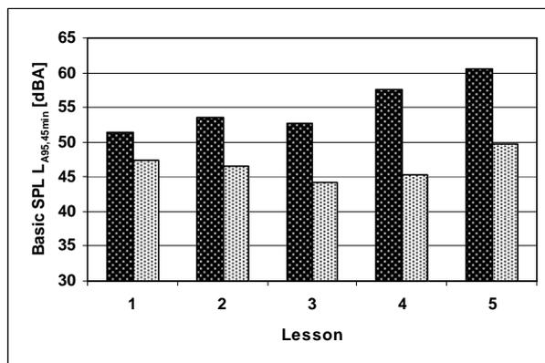
Figure 6: Mean Basic SPL LA95,45min before (▨) and after (▩) acoustical renovation
