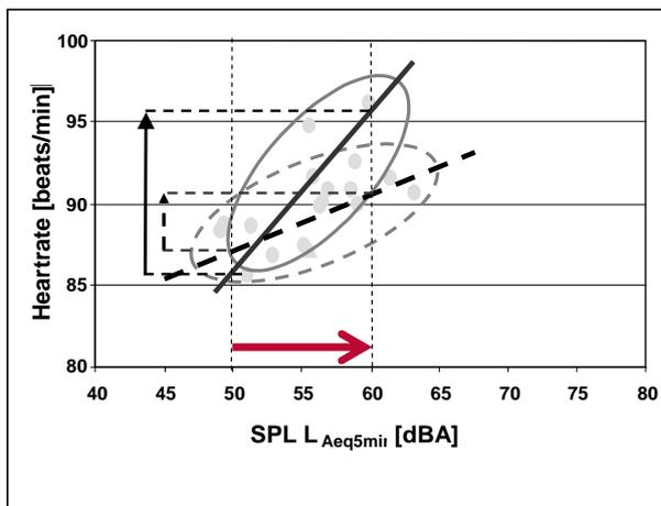
Figure 9: Heart rate reaction on noise before (—) and after (- - -) acoustic refurbishment of classroom
